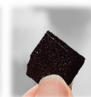
1 : Composite biobased powder ; 2 : Printing with a laser (SLS) ; 3. Printed material by SLS
